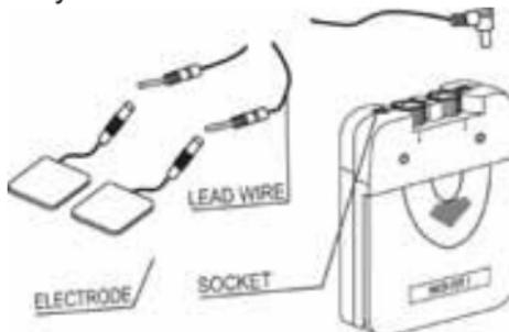
After connecting the wires to the stimulator, attach each wire to an electrode. Take care when you attach and detach the wires. Jerking the wire instead of holding the insulated connector body may cause wire breakage.
